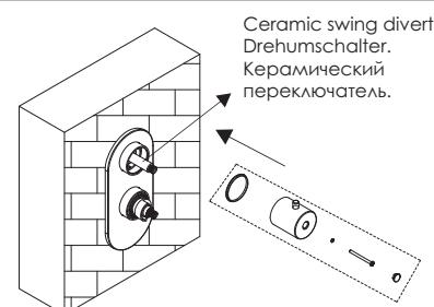
10. Adjust the black line to match with the mark on the cartridge.
